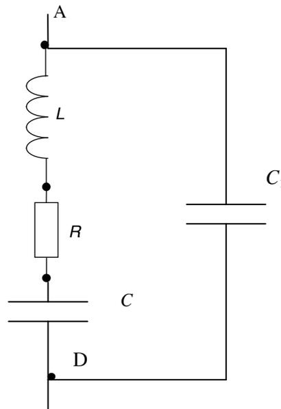
On donne :  $R = 9,0 \Omega$  ;  $L = 0,20$  H ;  $C = 10 \mu\text{F}$  ;  $U_e = 20$  V et  $C_1 = 2,0$  mF
